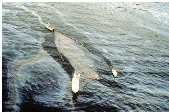
FIGURE 8.3 Oil boom in V configuration guiding oil to a skimmer [3].
